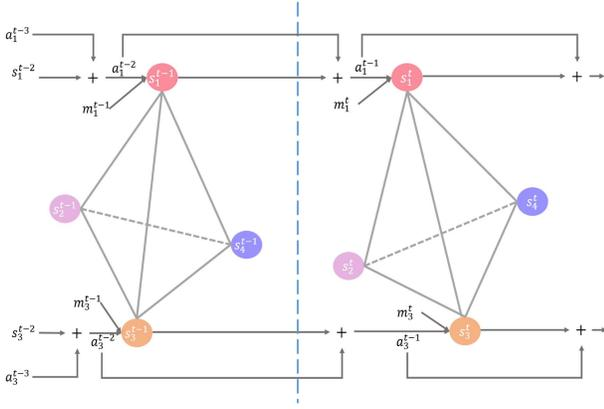
Fig. 4. The illustration of the proposed structure and updating mechanism of the fully-connected skip graph neural network. The nodes  $s$  are updated by the passing messages  $\eta$  and input features  $a$  in a recurrent way. The skip connection means the connection between  $a^{t-1}$  and  $a^t$ .
