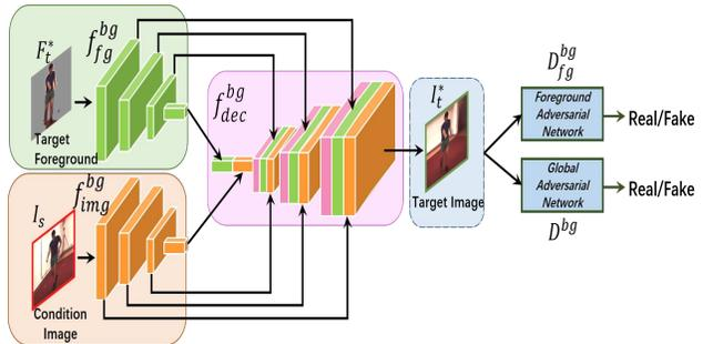
Figure 5. The architecture of the background transformer network.
