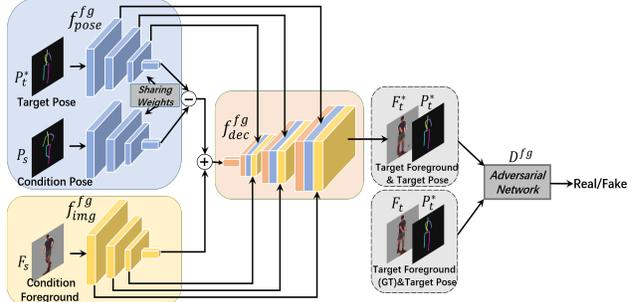
Figure 4. The architecture of the foreground transformer network.
